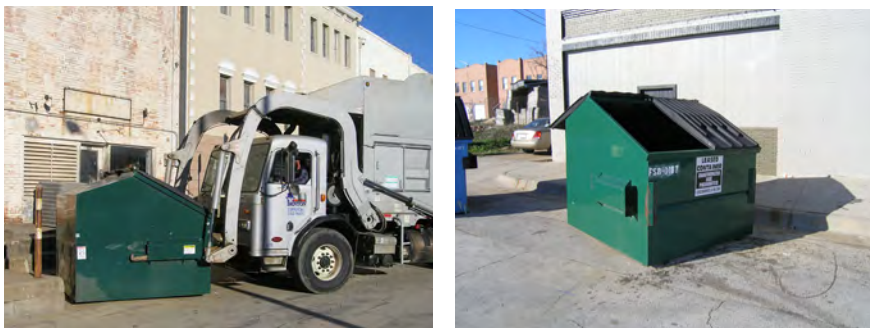
Front load container and truck Photograph 5.7
